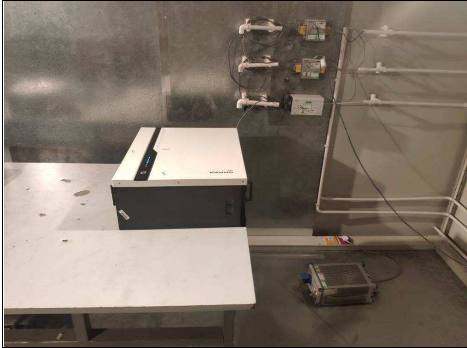
CONDUCTED EMISSION TEST (TELECOM PORT)
